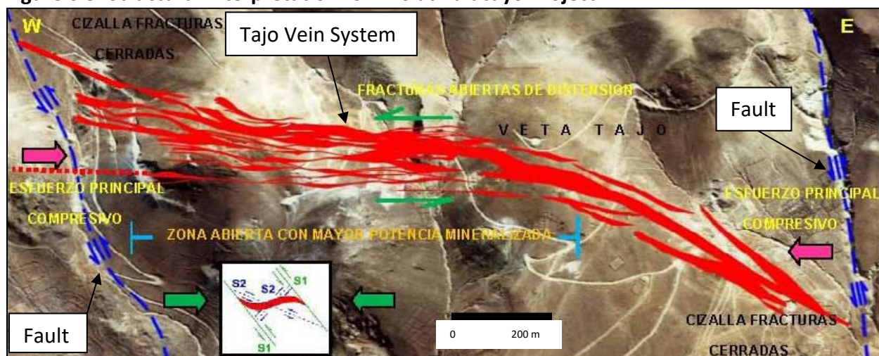
Figure 6.5: Structural Interpretation for TVS at Pulacayo Project
