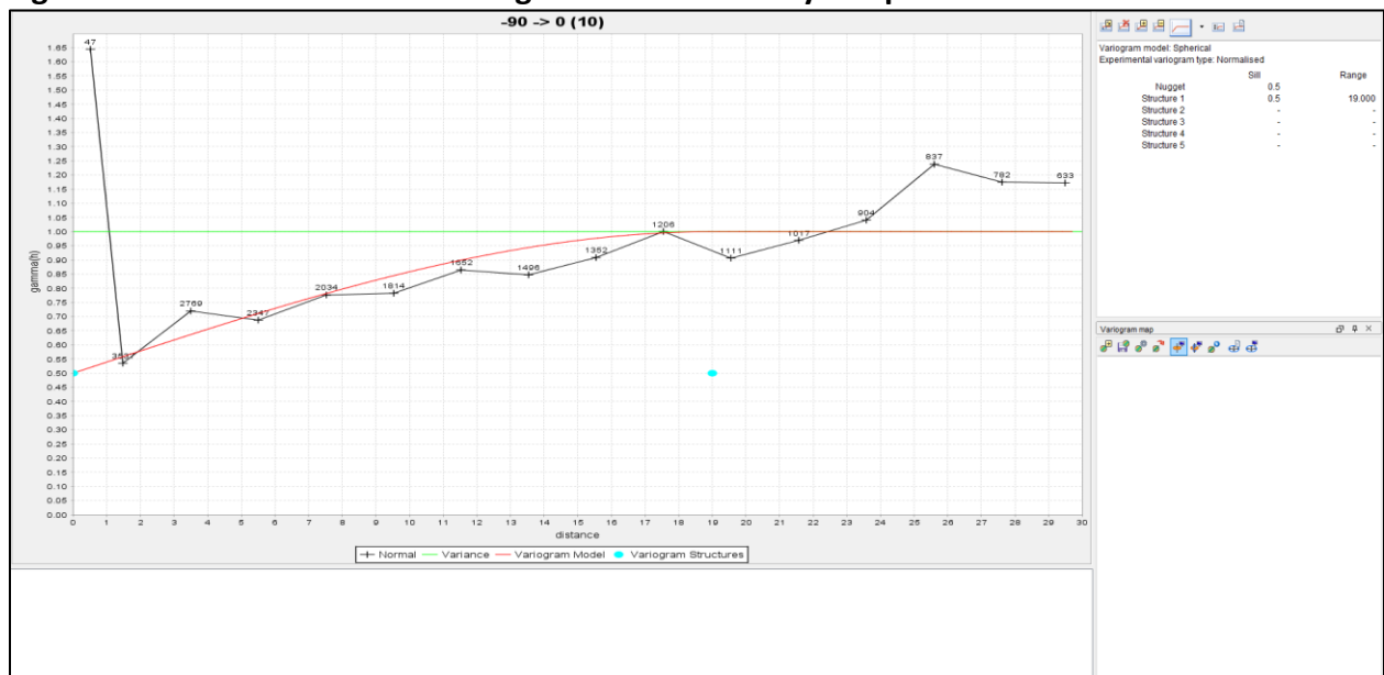
Figure 11.15: Downhole Zinc Variogram for the Pulacayo Deposit
